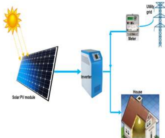
Fig. 2. Grid tied/direct PV system.
