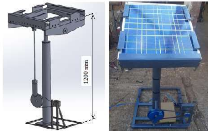
Fig- 11 (a) Model tracker; (b) Manufactured prototype
